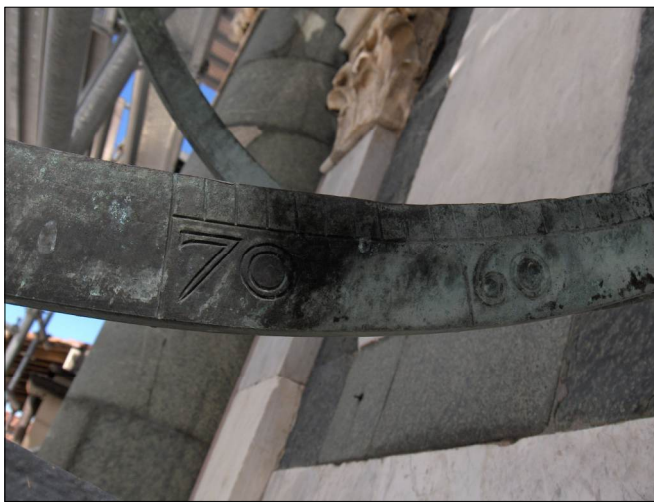
Fig. 11. Part of the graduation engraved on the meridian ring of the Armilla.
