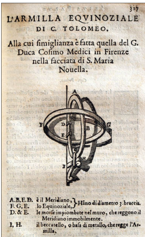
Fig. 1. A drawing of the Equinoctial Armilla as described in the 'Primo volume dell'uso et fabbrica dell'astrolabio', page 317.
