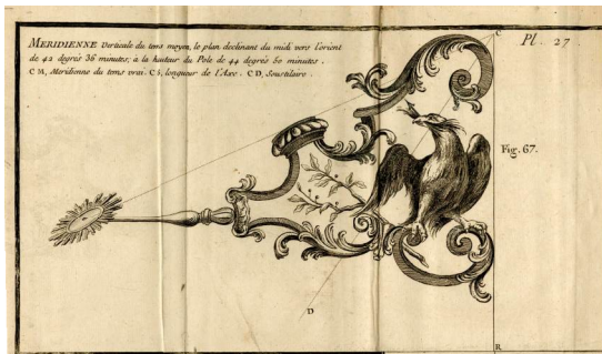
Fig. 4. Bedos de Celles: plate 27—vertical declining mean time noon dial.
