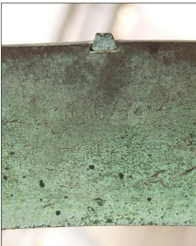
Fig. 7. The details of the slot carved in the convex part of the Equinoctial ring.
