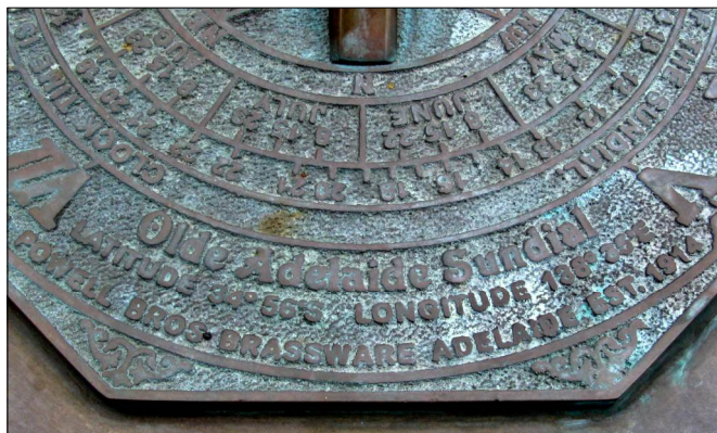
Fig. 5. Detail: Olde Adelaide Sundial, Latitude 34° 56' S Longitude 138° 35' E, Powell Bros Brassware Adelaide Est. 1914. Clock time is found by adding the minutes opposite today's date to the shadow reading of the sundial.
